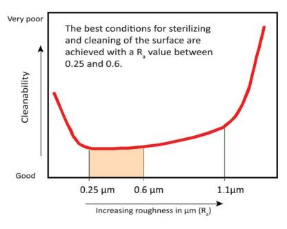
Figure 2. The cleaning of stainless steel is best done with a roughness of between 0.25 and  $0.6 \mu m$  (source Leser Hamburg).
