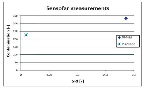
Figure 10: Contamination measurements SRI vs. Ra (source TNO)
