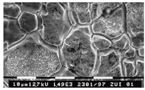
Figure 1. Pickled stainless steel AISI 316 (V=1500x) whose grain boundaries are affected preventively (source Dockweiler).
