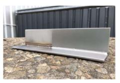
Figure 4. The right half is treated with the PureFinish process (photo Rösler).
