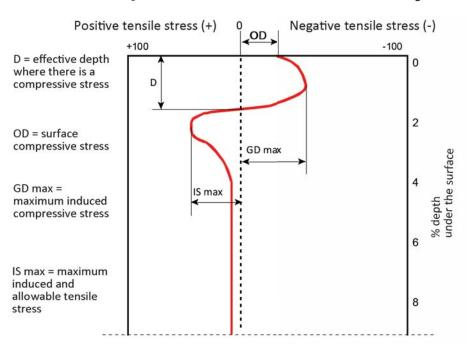
Figure 6: Schematic representation of pressure build-up on the surface.
